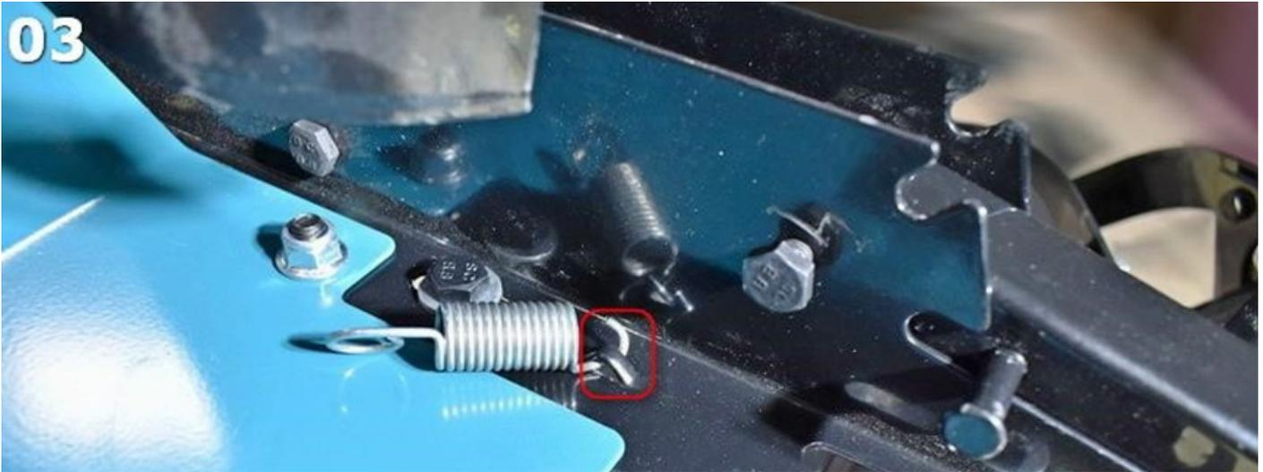
Use the pliers to grab the other end of the spring and fasten it to the special mounting screw on the transport wheel, as shown in fig. 4.
