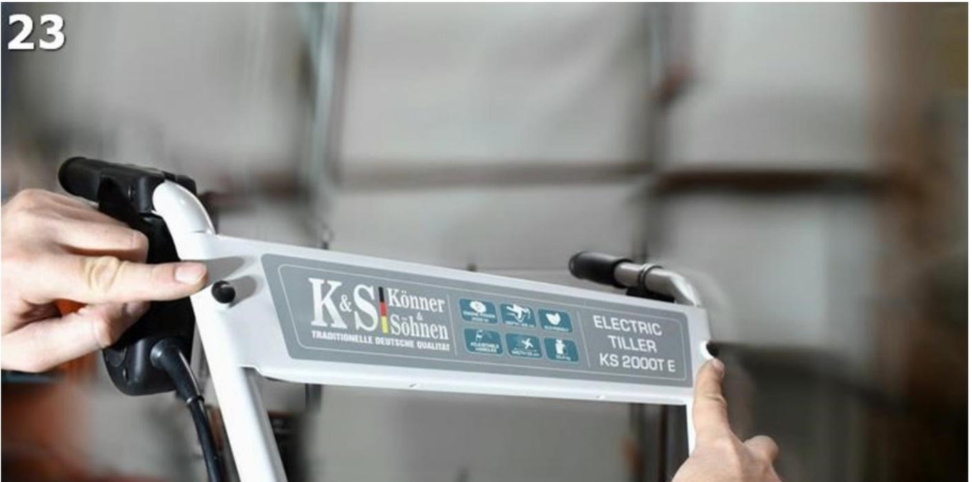
Before you start the engine, be sure to plug the cultivator into a power outlet. Press and hold down the blue button while lifting up the blue lever, as shown in fig. 24.
