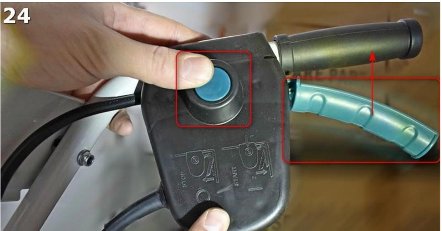
To set the cultivator in motion, pull the safety handle (1) on the clutch handle down and lift the clutch handle (2) up, as shown in fig. 25.
