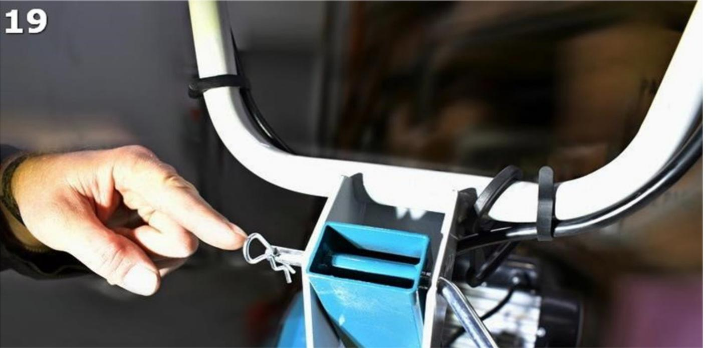
Fix the control panel in the lower position with the bolt, as shown in figs. 20 and 22.
