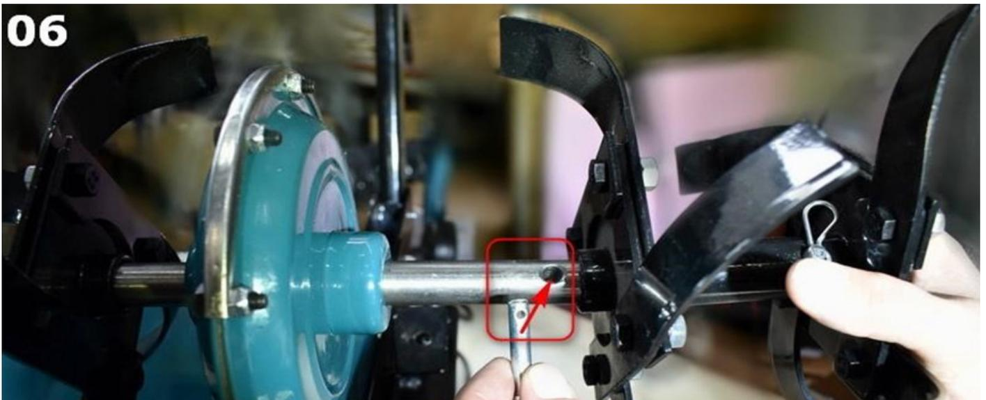
Secure the locking bolt with a cotter pin, as shown in fig. 7.
