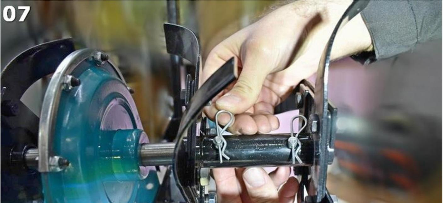
Put on the protective side disc, as shown in fig. 8.
