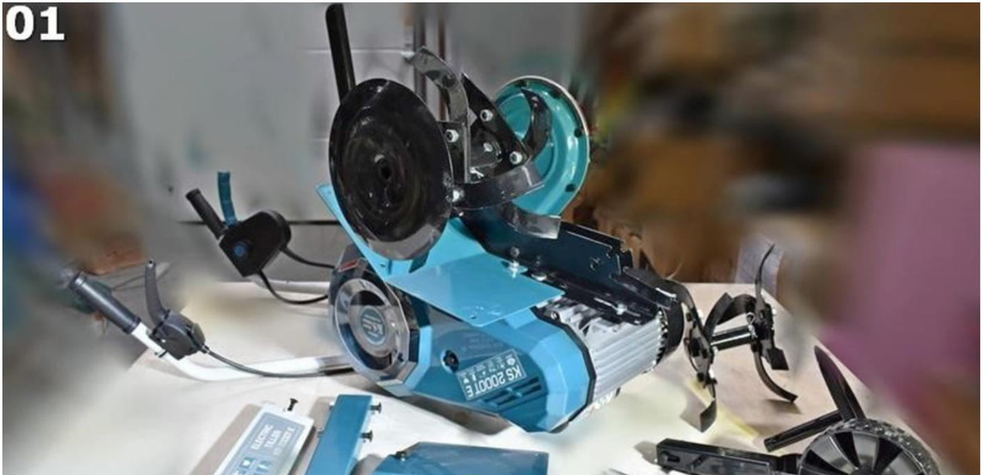
Proceed with assembly of the transport wheel. Attach the transport wheel to the cultivator body using the screw (1), as shown in fig. 2. Install the spring (2).
