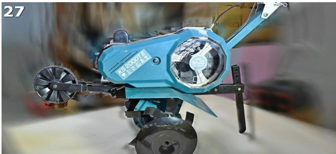
Be sure to adjust the coulter to the desired tilling depth, as shown in fig. 28.
