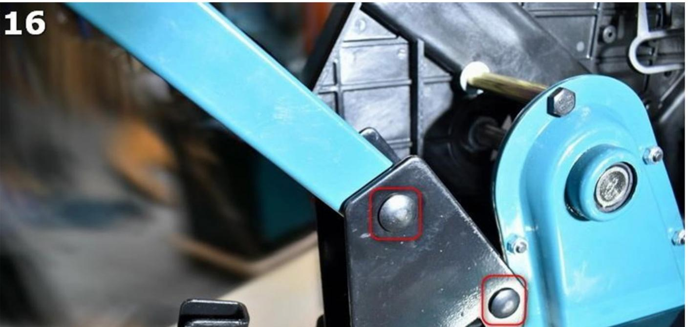
Install the operator's control panel using the bolt and locking bolt with cotter pin, as shown in fig. 17
