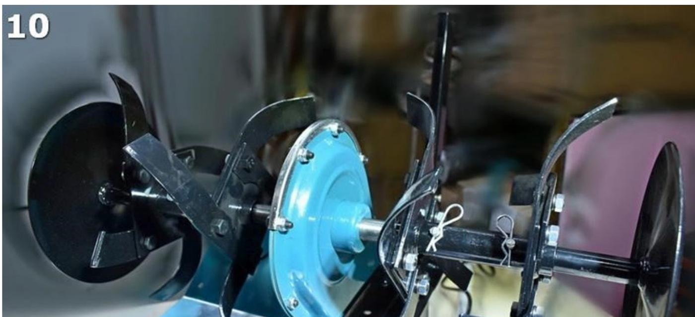
Adjust the coulter according to the desired tilling depth. Fix the coulter with the locking bolt and cotter pin, as shown in fig. 11.
