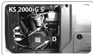
For all modifications of models KS 2000i, loosen the 4 screws on the side panel. Loosen drain screw **C** on the carburetor and let the remaining fuel drain through pipe **D** into the dedicated drip pan. Avoid gasoline leaks. Tighten up the screw. Install back the generator housing cover. Start the generator on LPG.
