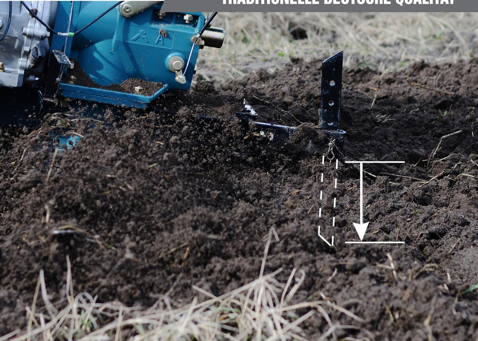
3. Gradually increase the tilling depth when cultivating soil, for which purpose apply pressure on the steering wheel to increase the coulter depth.
