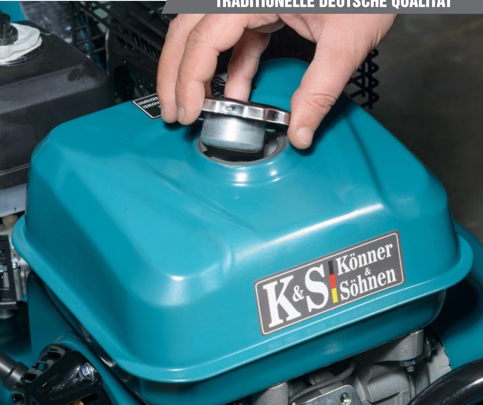
3. Fill the fuel tank with gasoline.
