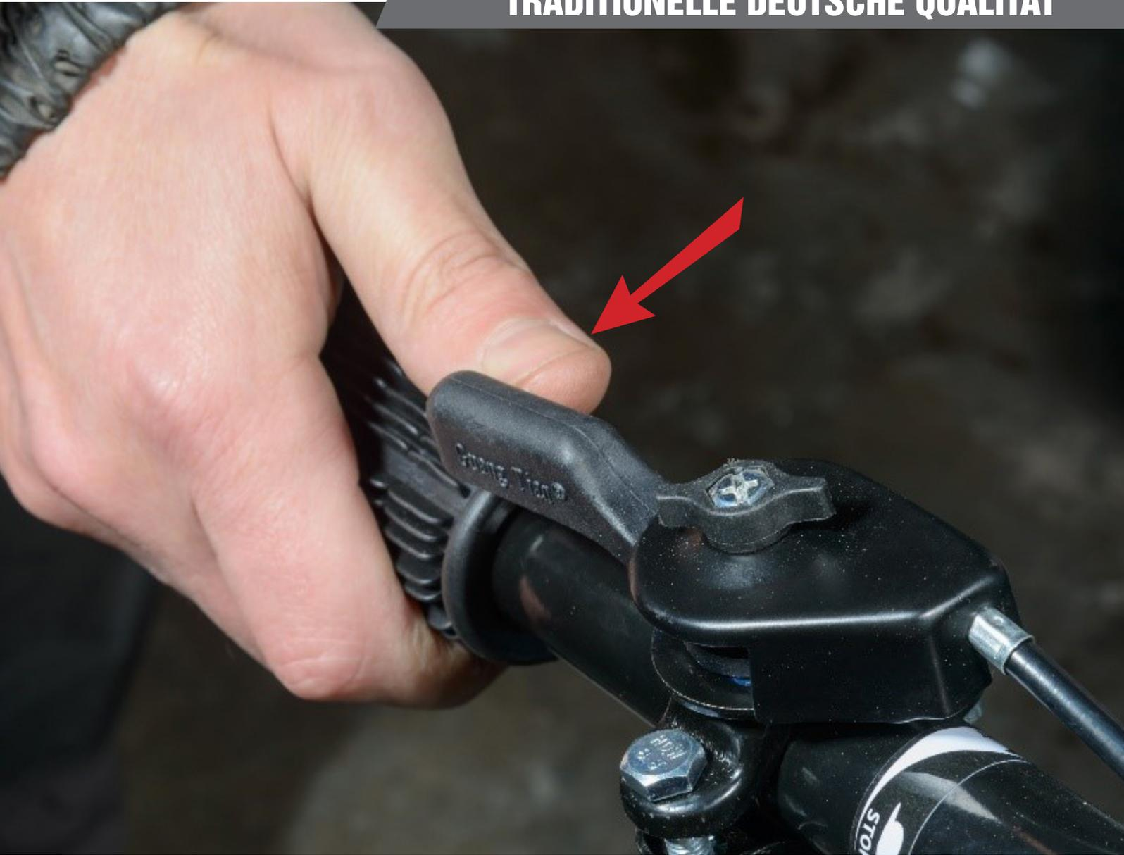
3. Turn the engine speed control to “MAX”.
