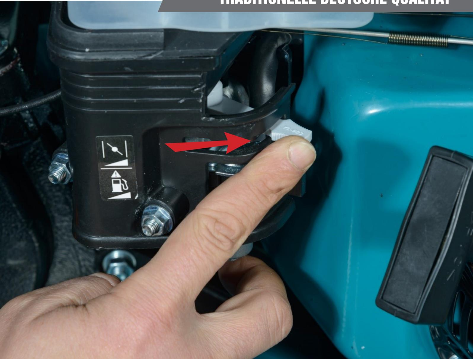
8. After the engine has started, turn the air choke control knob to “Open”.
