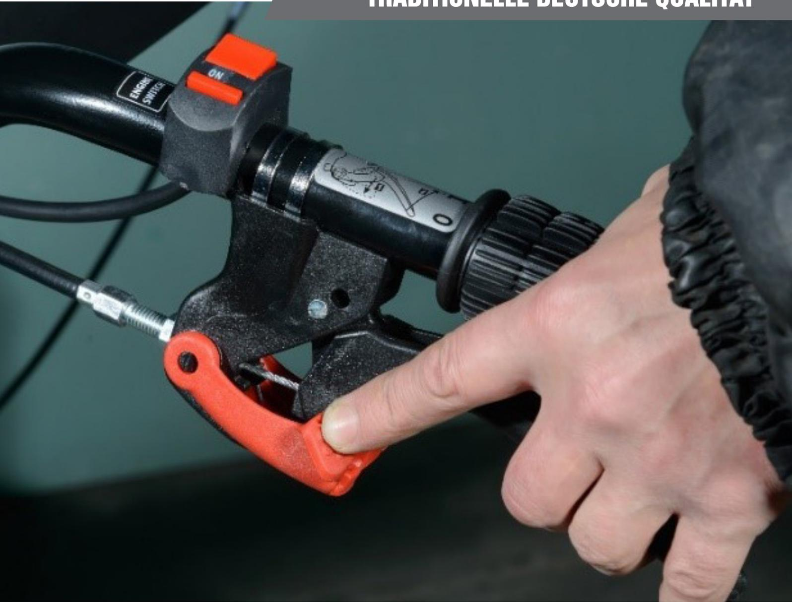
2. Press the red fuse (near the clutch lever), press and hold down the clutch lever.
