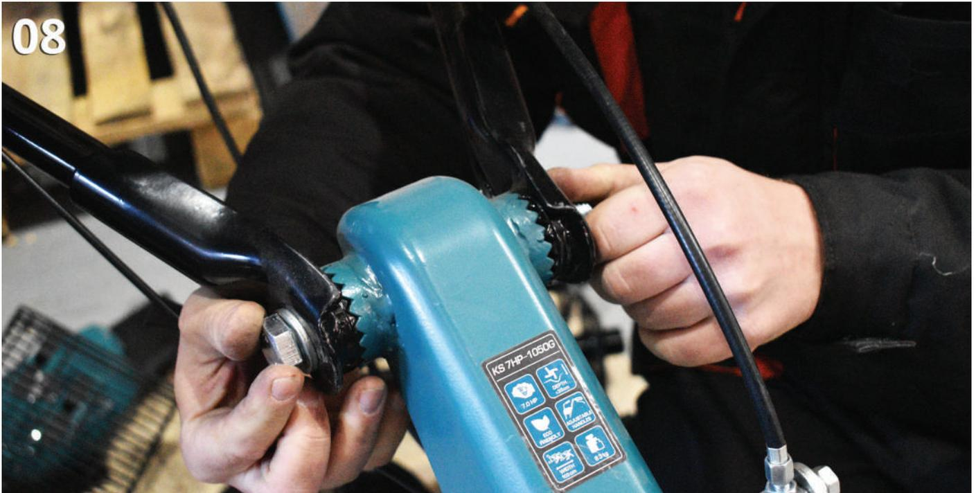
Fig. 9. Lock the position of the handlebars with the clamp fixture.
