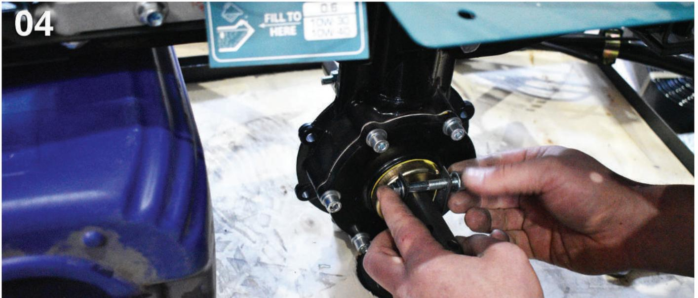
Fig. 5. Install the plow holder mount on the cultivator frame with the locking pin. Secure the locking pin with a cotter pin.
