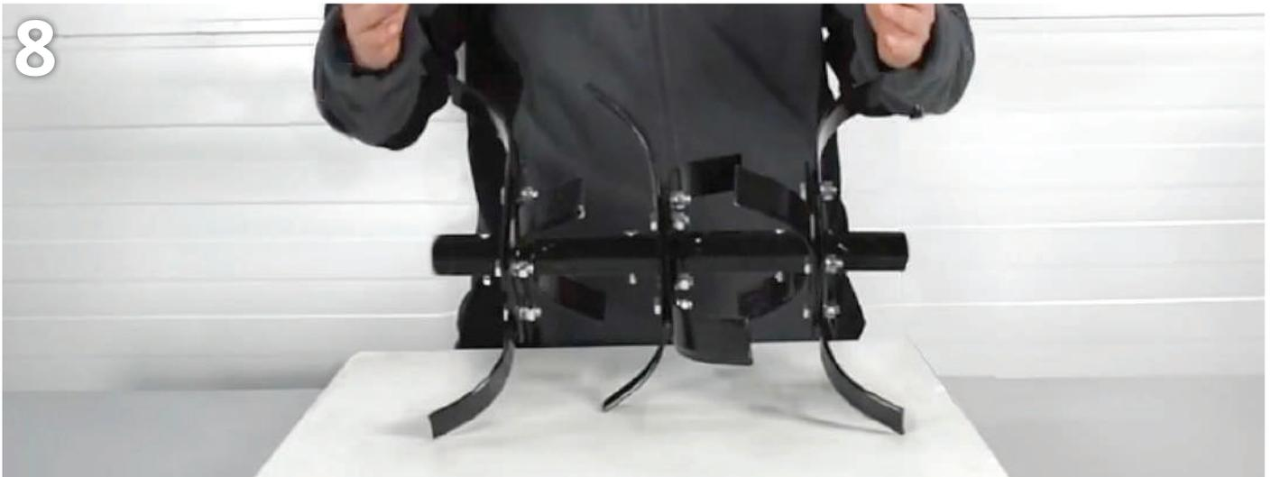
Fig. 9. The right cultivator cutters are mounted inversely. The cutting edge of the knives should be at the front in the direction of travel of the cultivator.
