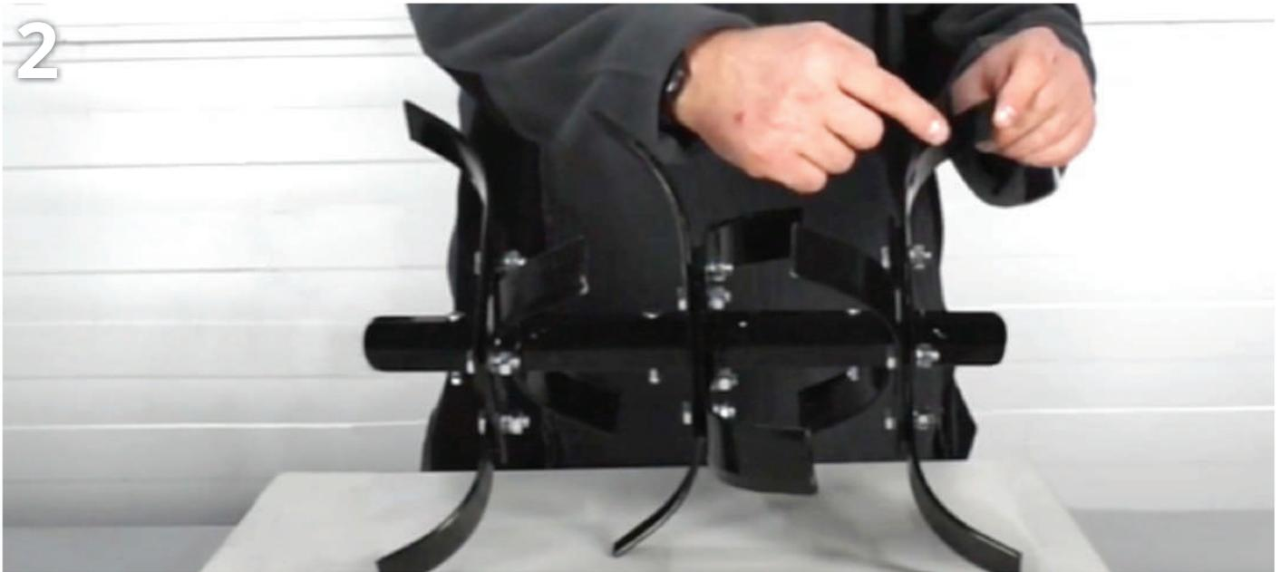
Fig. 3. Assemble the cultivator's left cutters. The left knives have their cutting edge against the user pointing to the left, with the right knives having their cutting edge against the user pointing to the right.
