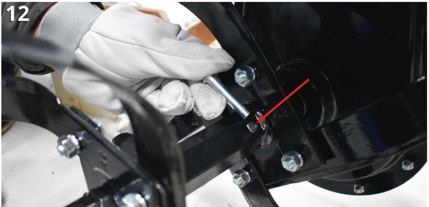
Fig. 13. Secure the fender to the cultivator with bolts and nuts.
