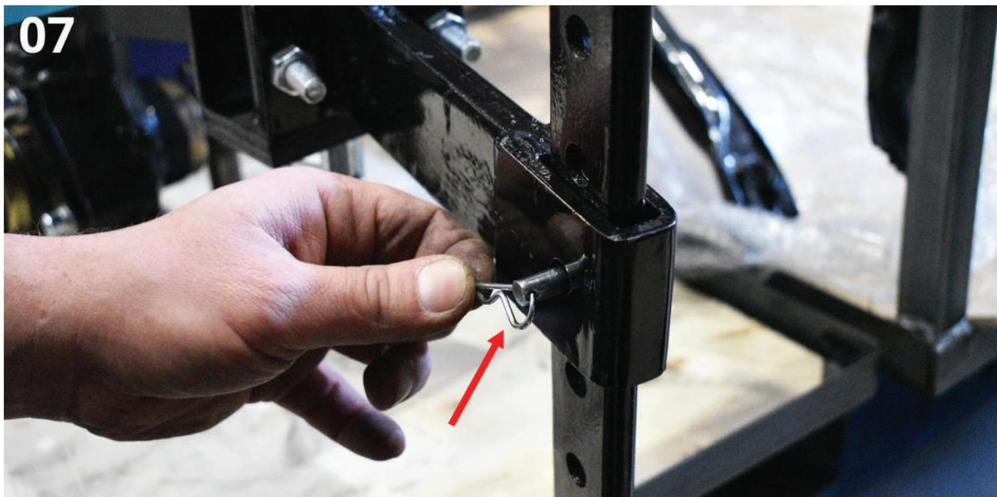
Fig. 8. Adjust the tilt angle of the control handle.
