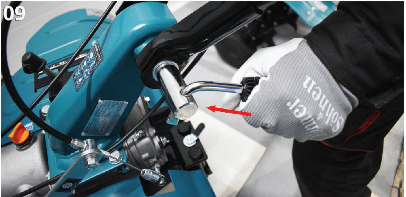
Fig. 10. Pass the screw through the clutch spring eyelet.
