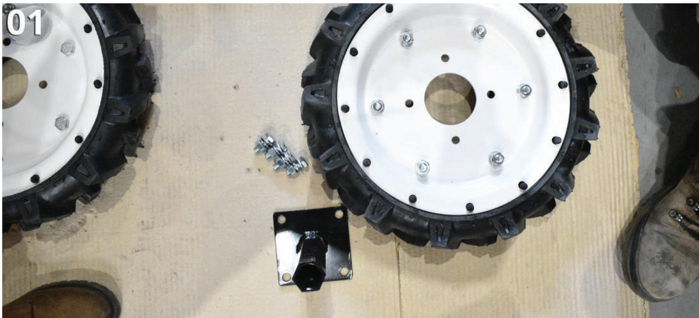
Fig. 2. Secure the transport wheel to the axle using bolts, nuts and washers.
